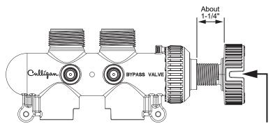
A screwdriver shank may be used in the slot as a lever for extra turning force if needed
