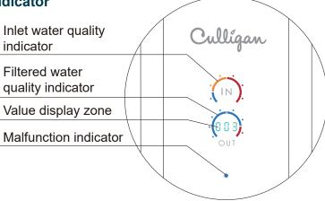
Figure 1. Front Cover Indicator Lights
