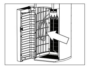
1. If installing a filter, locate the coil of tubing inside the cabinet on the left side.
