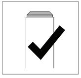
**IMPORTANT:** The in-line strainer must be fully seated into the water line or else the line will leak. The in-line strainer has a tight fit and may be difficult to push back into the water line.
