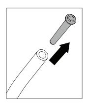
3. When clean, install the strainer back into the water line. Be sure to seat the strainer properly or the line will not be sealed properly and will leak.
