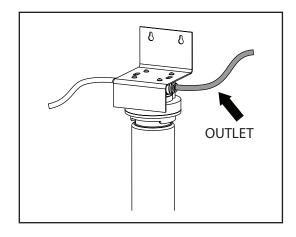
2. The **blue** tube must be connected to the filter system outlet.
