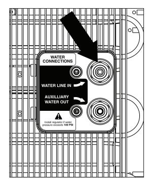
4. Insert the filtered water out line (blue) into the Water Line In bulkhead fitting on the back of the unit.
