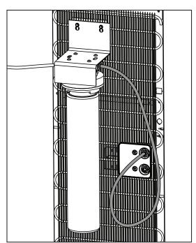
3. Mount the filter to the condenser coils on the back of the unit high enough that the filter can be removed.
