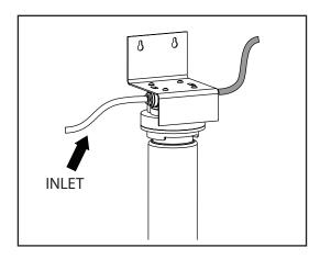
1. The **white** tube must be connected to the filter system inlet.
