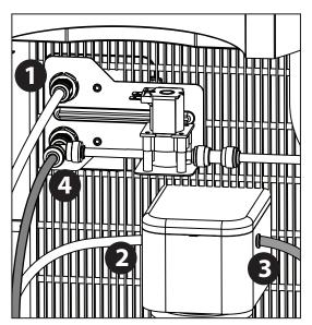
4. Connect water inlet line (white) (1) to the inlet fitting on the filter head (2). Connect water outlet line (blue) to the water outlet fitting on the filter head (3) and connect to the tee fitting (4).
