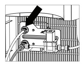
The in-line strainer is located inside the cooler and set into the water line-in tubing (white) in the top bulkhead fitting.
