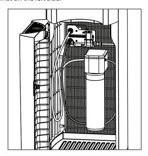
3. Mount the filter to the condenser coils inside of the unit high enough that the filter can be removed.
