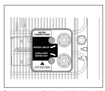
To connect to a water line, locate the inlet on the rear of the unit and remove the plug from the push-to-connect fitting marked "Water Line In".
