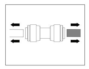
2. Disconnect and remove the push fit union fitting and use the tube ends to connect to the filter. (see Fig. A)
