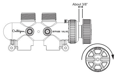
Figure 1. Bypass Position.
